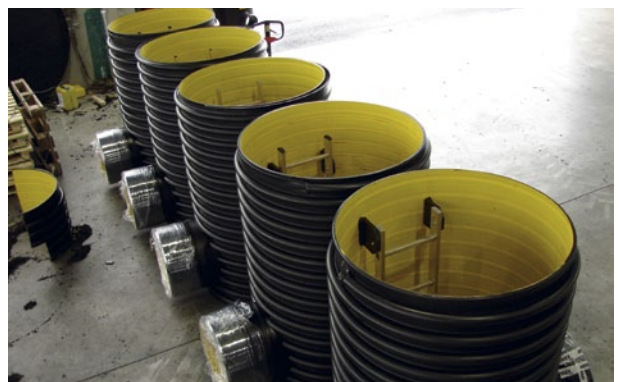
Rainwater manholes with electro-fusion fittings
