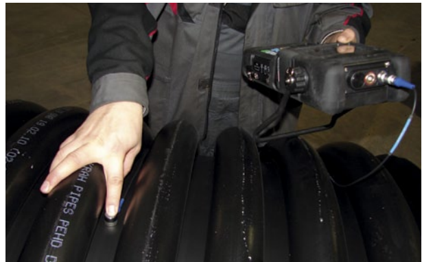
Measuring the width of the pipe wall
