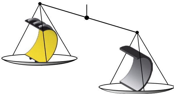
By using profiled pipes we can save weight up to 65% compared to equivalent solid wall pipes with the same static capacity.
