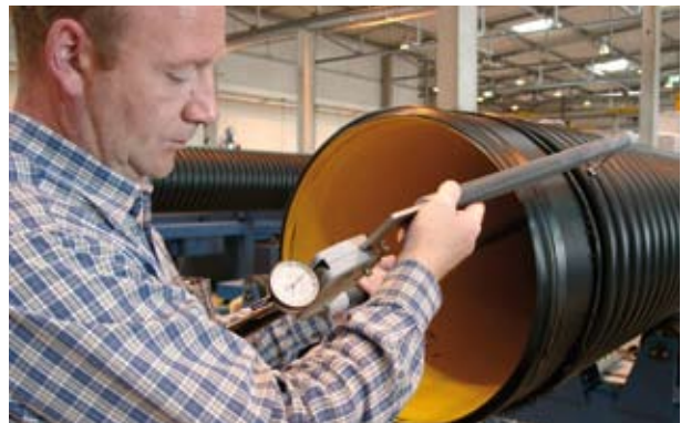
Checking of the wall thickness
