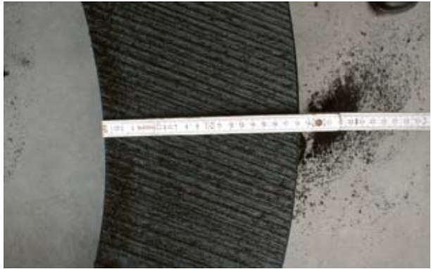
Solid wall polyethylen pipe, s = 180\text{mm}
