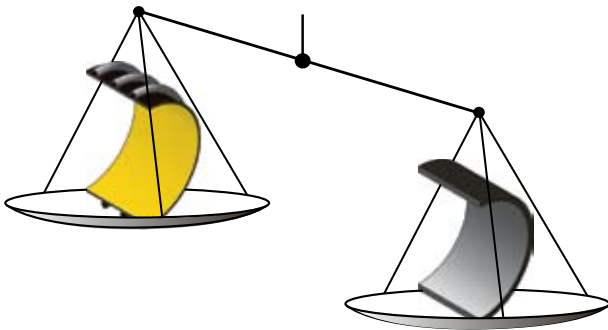
By using profiled pipes we can save weight up to 65% compared to equivalent solid wall pipes with the same statical capacity.
