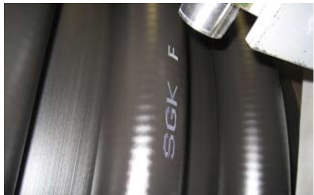
Marking of a pipe
