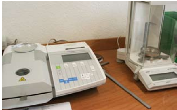
MFR-testing and moisture testing
