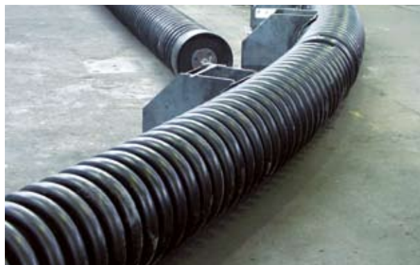
Bending of Krah pipes R/D = 30
