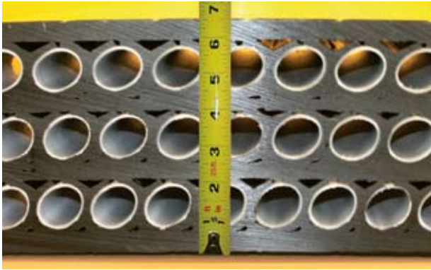
Wall of a SQ pipe
