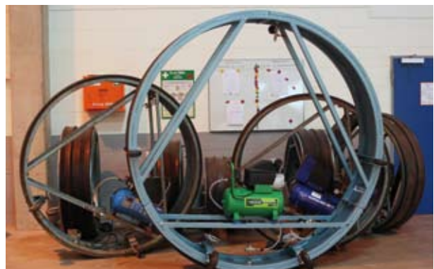
Devices for leak tightness test of joints
