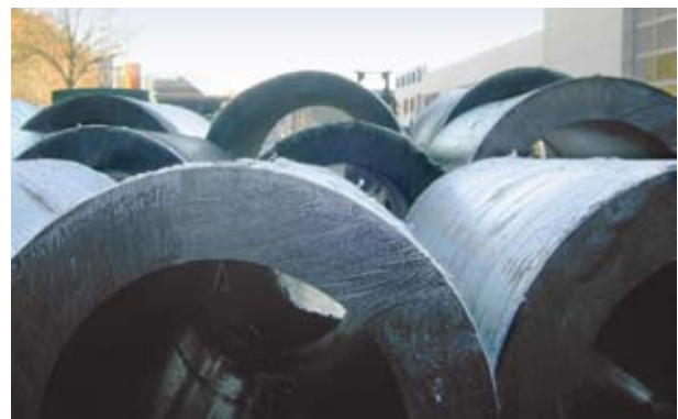
Heavy wall pipes DN/ID 500mm, s = 140mm
