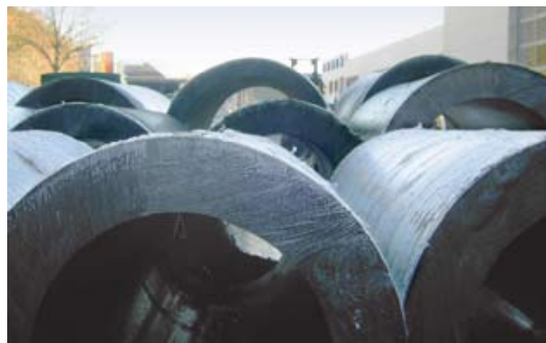
Paksuseinalised torud DN/ID 500 mm, s = 140 mm
