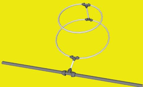
The system enables a unique below-surface, adjustable, even waterflow distribution through the insertion of a customizable drip-irrigation pipe into the system, which can be adapted according to the tree pit's dimensions. The irrigation system's sub-surface positioning protects the mechanism from vandalism.
